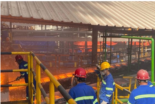
NPI being poured into an Ingot caster
