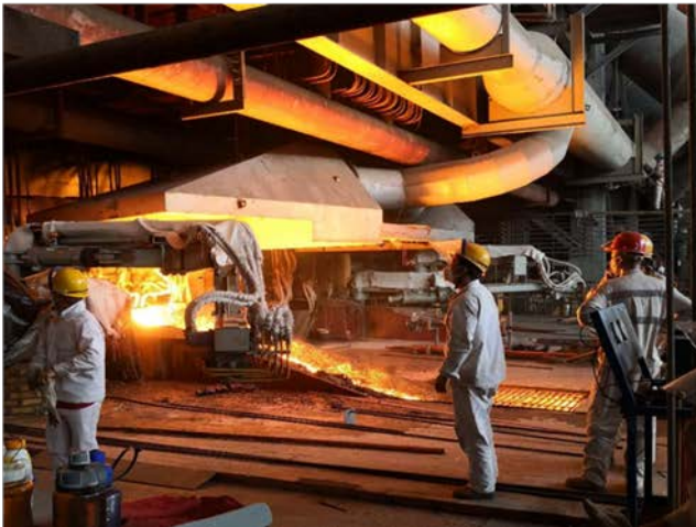
Ranger Nickel's first production run showing the flow of molten NPI
