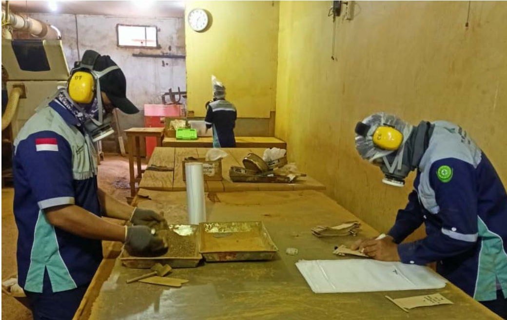
Photo 12 -3mm sample, manual incremental reduction JIS M 8109-1996
