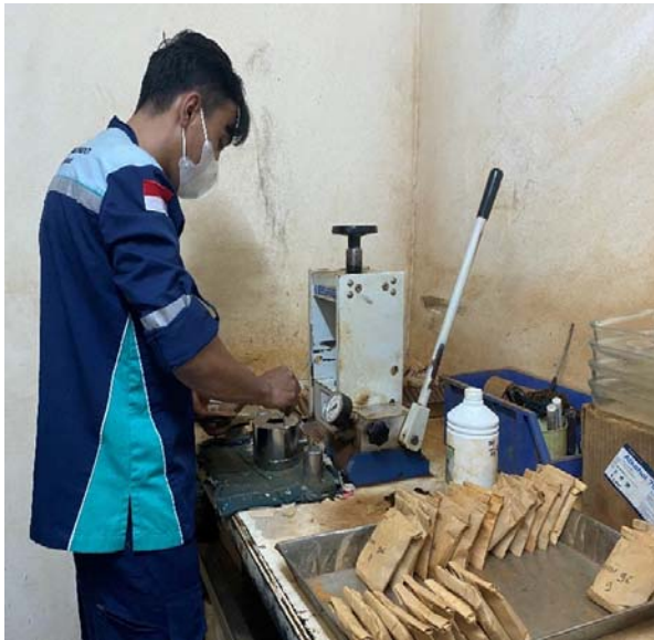
Photo 26 Pressed pellet production from sample pulp ready for XRF analysis
