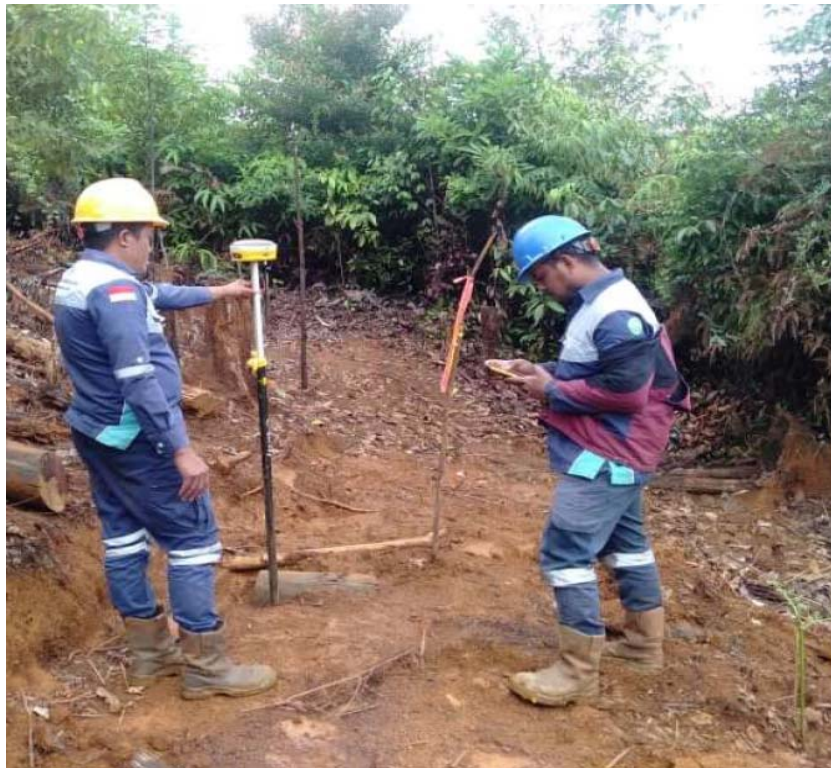
Photo 4 Drill collar survey using E-survey RTK GPS
