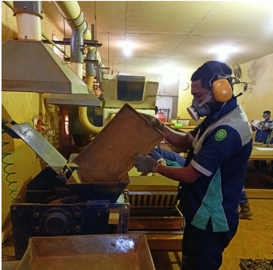
Photo 11 Jaw crushing to -10mm
