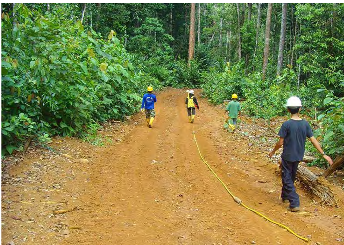
Photo 4-1 Ultra GPR survey acquisition (source: Groundradar.com)
