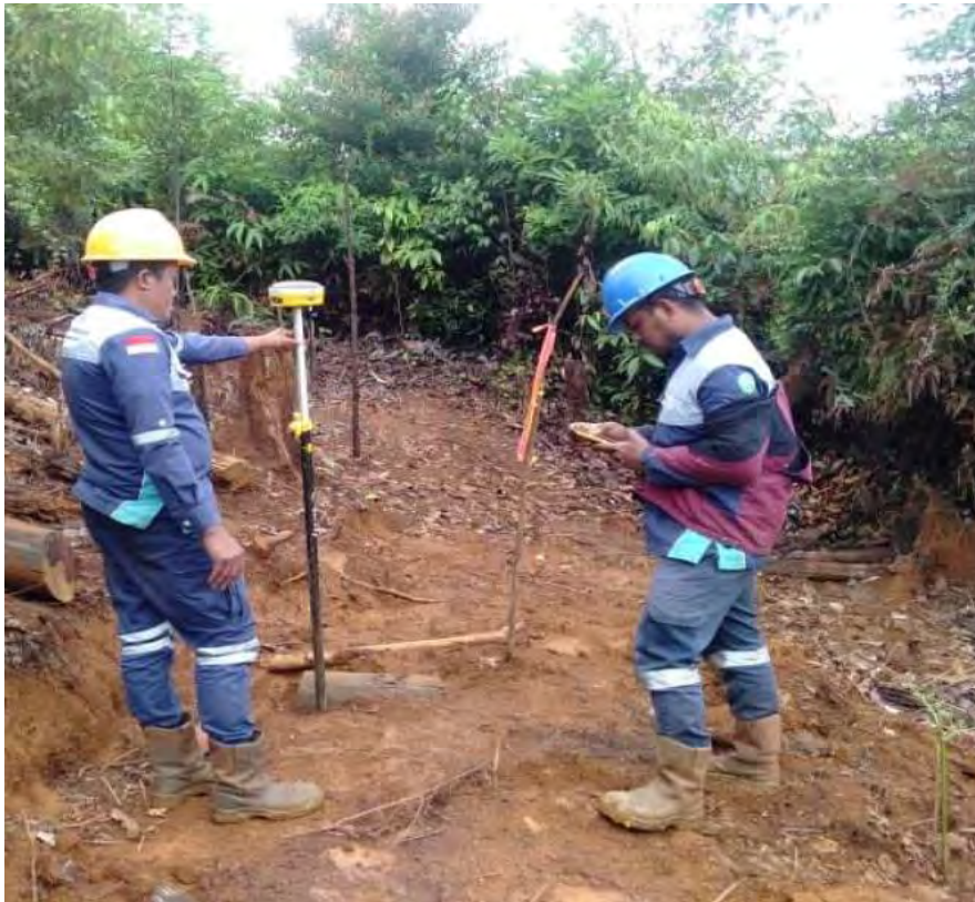
Photo 4-3 Drill collar survey using E-survey RTK GPS
