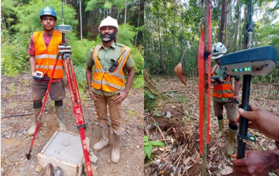
Photo 7 Drill collar survey at IMM
