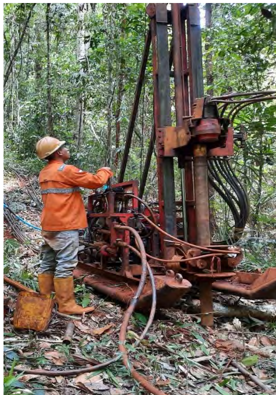
Photo 4 Dexdrill 200 operating at ETL
