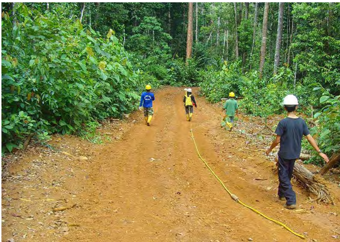
Photo 3 Example survey acquisition using UltraGPR (source: Groundradar.com)
