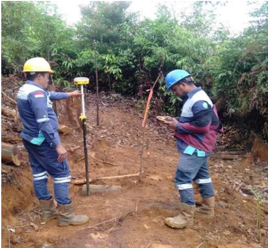
Photo 4-3 Drill collar survey using E-survey RTK GPS
