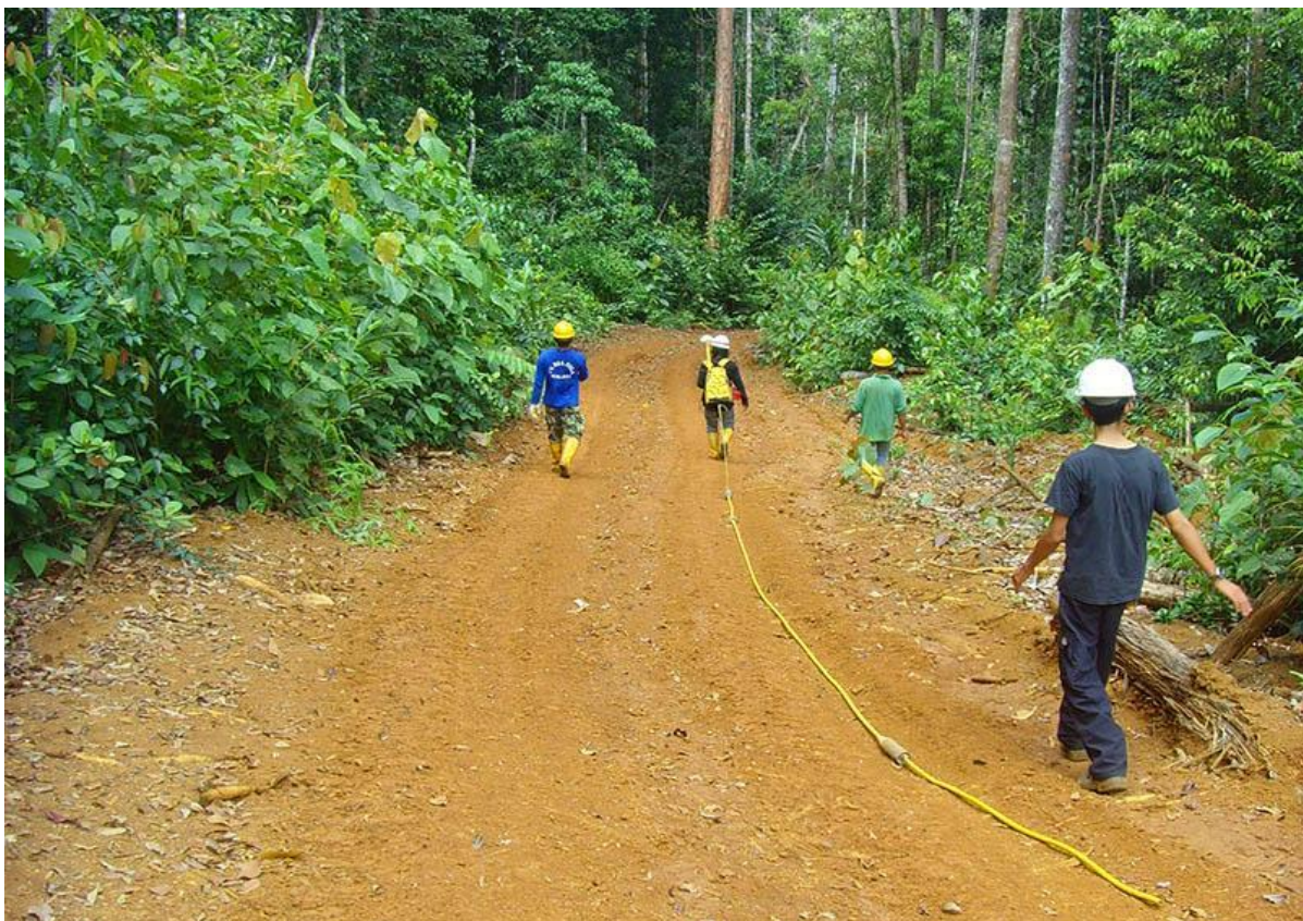
Photo 4-1 Ultra GPR survey acquisition (source: Groundradar.com)
