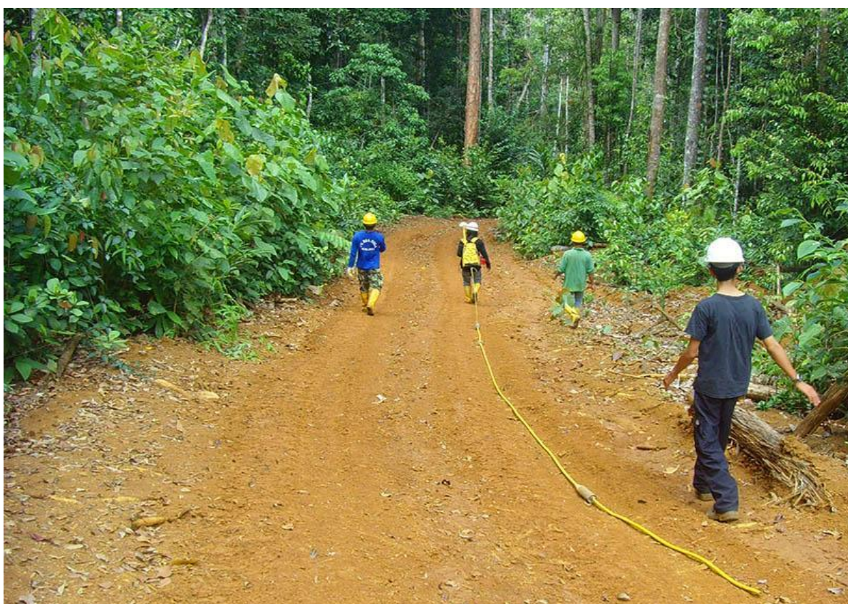
Photo 4-1 Ultra GPR survey acquisition (source: Groundradar.com)
